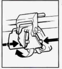
Lower the sun visors and push both sides of the lock buttons on the front latches.
