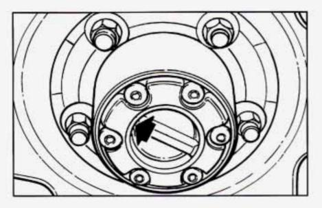
To unlock the hubs, turn the hub dials to FREE.
