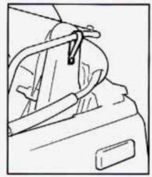
Fasten the upper top bow with the belt on the driver's side seat belt shoulder anchor bracket.
