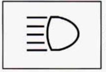
When the high beams are on, a light on the instrument panel also will be on. It will go off when you switch to low beam.
