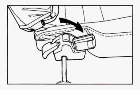
Pull the knobs on both sides of the seatback. If you have the split rear seat, you can fold half of the seat by pulling only the knob on the side you wish to fold.
