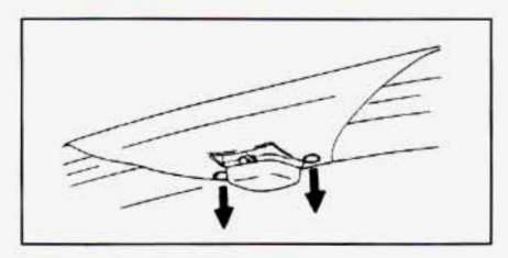
Unfasten the snaps that secure the canvas top to the roof piece. The snaps are located on either side of the dome lamp.
