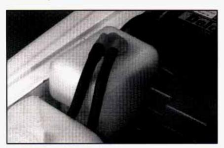
When your engine is cold, the coolant level should be at LOW, or a little higher. When your engine is warm, the level should be up to FULL, or a little higher.
