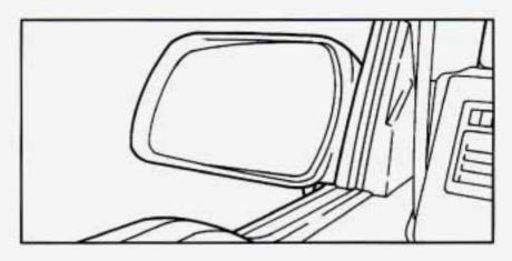
Adjust these mirrors by hand so that you can just see the side of your vehicle when you are sitting in a comfortable driving position.
