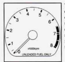
The tachometer shows engine speed in thousands of revolutions per minute (rpm). You can use it while driving to select correct shift points. The tachometer may not return to zero when the engine is not running.
