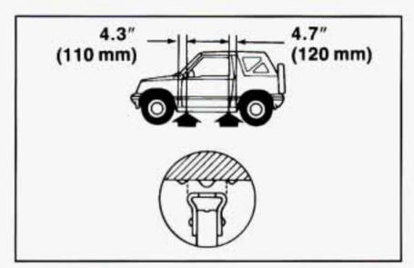
Position the jack and raise the jack lift head until it fits firmly onto the notches nearest to the flat tire. (Under the vehicle near each wheel, there are notches in the vehicle's rocker flange.)
