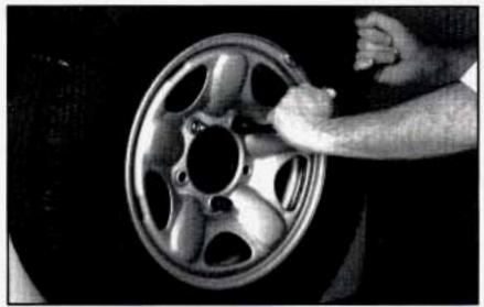
Remove wheel nuts with the wheel wrench.
