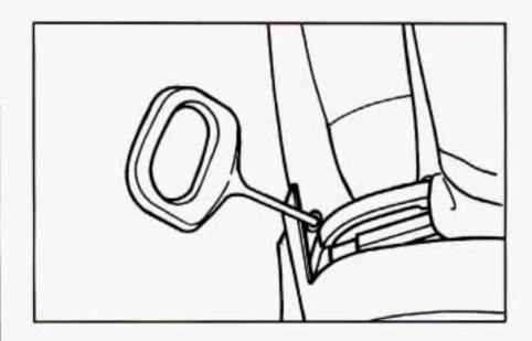
To get out, pull the release handle on the rear of the passenger's side front seat.
