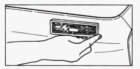
Push the sidemarker housing toward the back of the vehicle to release the clip and pull out the front edge. The housing should pull away from the vehicle.
