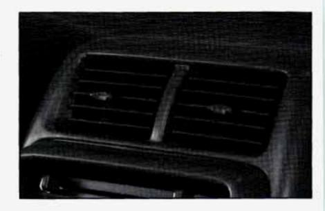
Your vehicle has air outlets that allow you to adjust the direction and amount of airflow inside the vehicle.
