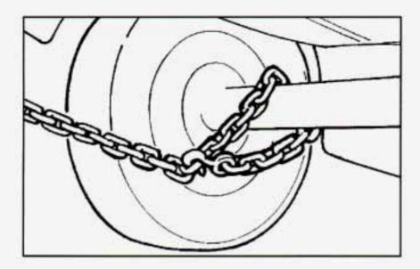
Attach a separate safety chain around the end of each axle, inboard of the spring.
