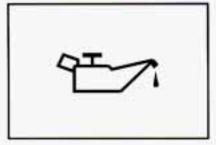
If the engine oil pressure light on the instrument panel comes on, it means you need to check your engine oil level right away.
