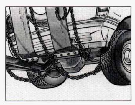
Position the sling crossbar under and forward of the rear bumper.
