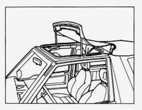
Swing the front top bow up and back while folding the canvas top out from between the top bow and the roof support. Be sure that you don't pinch the canvas top between the front top bow arms and the roof rails.
