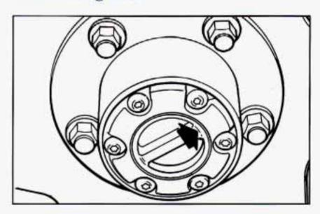
Your vehicle may have either manual or automatic freewheeling hubs. You must lock the hubs before you use FOUR-WHEEL HIGH (4H) or FOUR-WHEEL LOW (4L).
