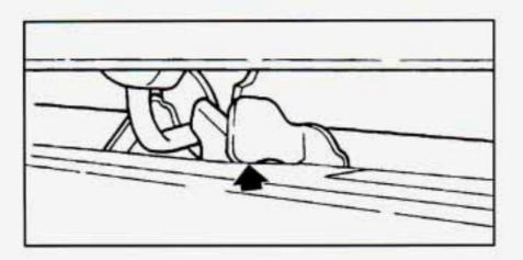
Then go to the front of the vehicle, pull up on the hood, and push the hood release lever to your left.
