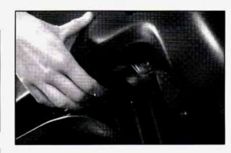
To open the hood, first pull the release handle inside the glove box.
