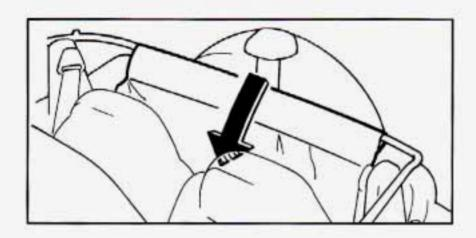
Lower the folded canvas behind the rear seatback(s). Make sure that the rear seat belts around the shoulder anchor are clear from the folded top.
