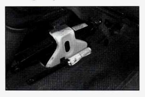
The jack and wheel wrench are under the front passenger's seat.
