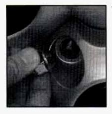
Replace the wheel nuts with the rounded end of the nuts toward the wheel. Tighten each nut by hand until the wheel is held against the hub.
