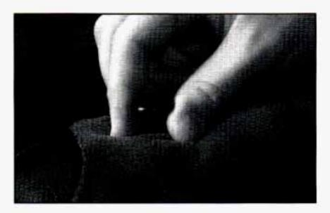
Pull up on the lock knob on the top of each seatback.
