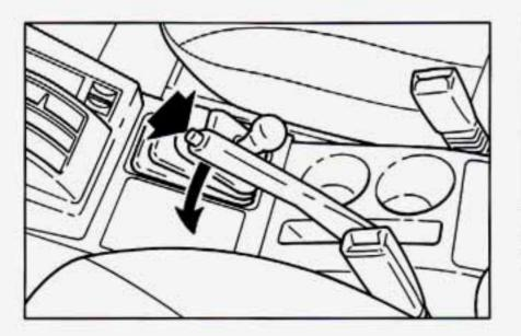
To release the parking brake, hold the brake pedal down. Pull the parking brake lever up until you can push in the release button. Hold the release button in as you move the lever all the way down.
