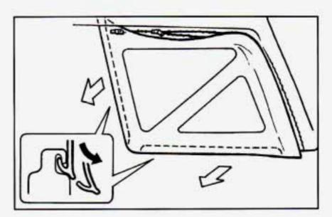
Unzip the zipper the rest of the way and remove the side window.
