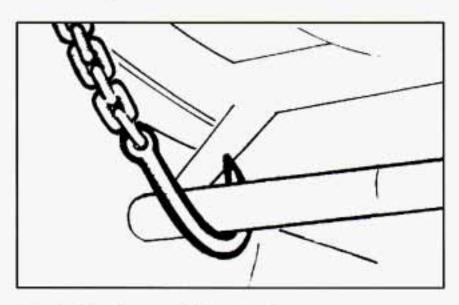
Attach J-hooks around the axle tube.
