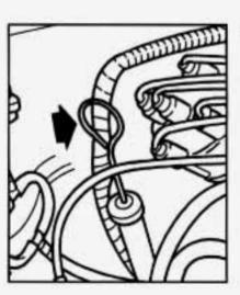
The automatic transmission dipstick is a black ring handle located in the rear of the engine compartment toward the passenger's side of the vehicle. Pull out the dipstick and wipe it with a clean rag or paper towel. Push it back in all the way, wait three seconds and then pull it back out again.
