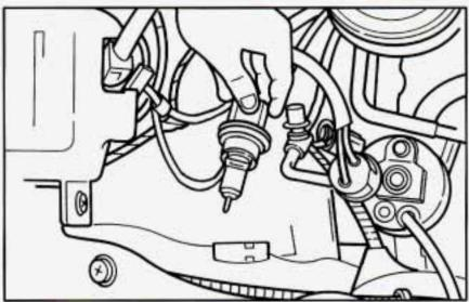
Turn the lock ring to the left to release the bulb.
