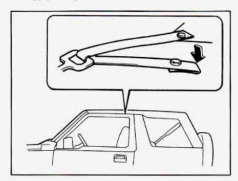
Unfasten the snaps on the driver's and passenger's sides of the roof side tension belts, located above the doors on the outside of the vehicle, underneath the canvas top.
