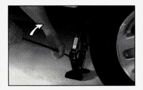
Raise the vehicle by turning the jack handle to the right. Raise the vehicle far enough off the ground so there is enough room for the spare tire to fit.
