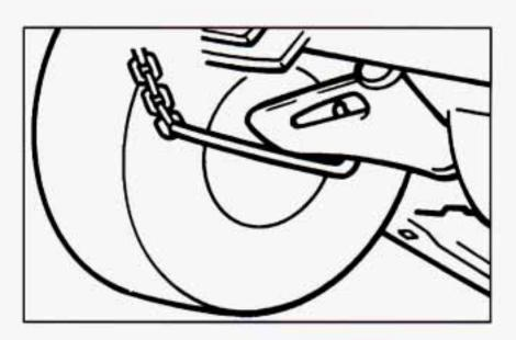
Attach J-hook chains on both sides to the rear of lower control arms inboard of the spring.
