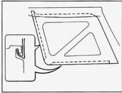
After completing installation, make sure that the front and bottom ends are securely hooked and the rear top end of the window is under the canvas top.
