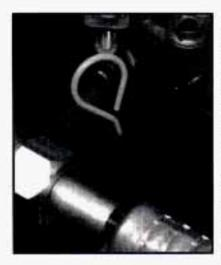
The engine oil dipstick is a yellow ring handle and is located near the front of the engine compartment toward the passenger's side of the vehicle.
