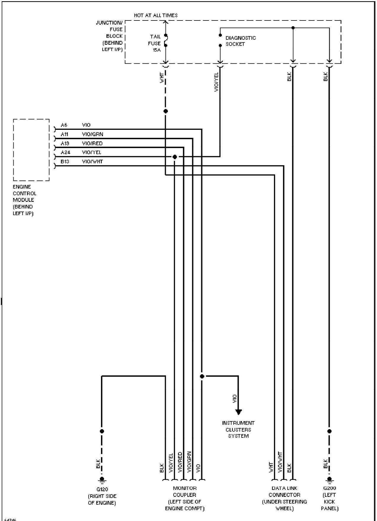
Data Link Connector Circuit
